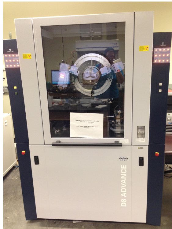
Figure B.4 Bruker D8 ADVANCE diffractometer with a \text{Cu K}\alpha ( \lambda = 0.154 \text{ nm} ) radiation source.
